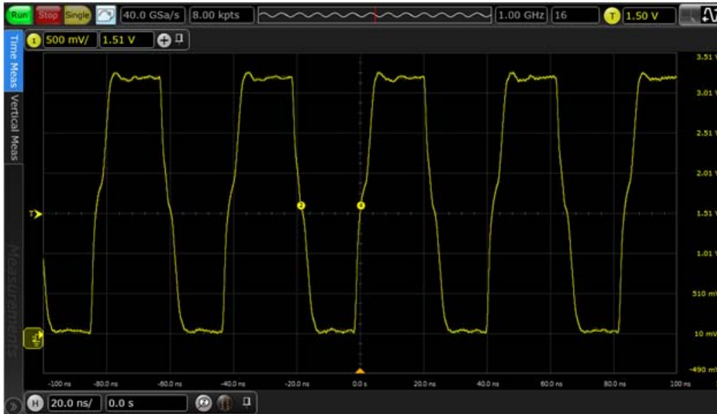
Figure 16. Correctly set DSE for 24 Hz signal (DSE = 37 \Omega SRE = low, SPEED = 50 MHz)
