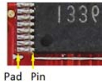
Figure 1. Pin and pad
